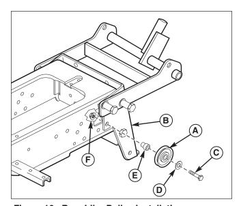
Figure 10. Rear Idler Pulley Installation
